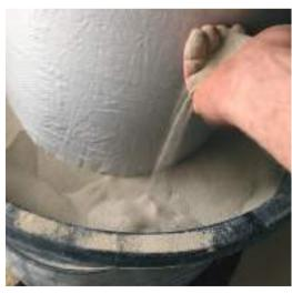
The basic material: finely powdered clay with a low moisture content
