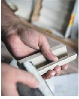
The plaster mould removes *moisture from the clay.* Once the material has dried, the border is removed from the mould and must be left to dry for three or four more days. Only then can it be fired.
