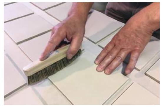
Before bisque firing the body is cleaned from dust.
