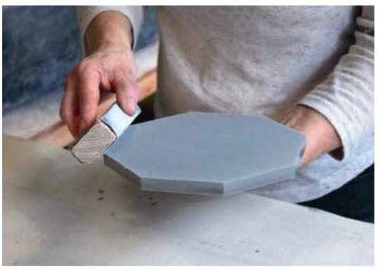
The edges of the blank are sanded down before firing.
