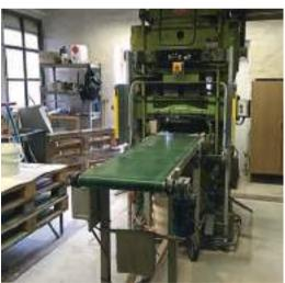
Dry press machine for the production of bisques Determining the right amount of glaze
