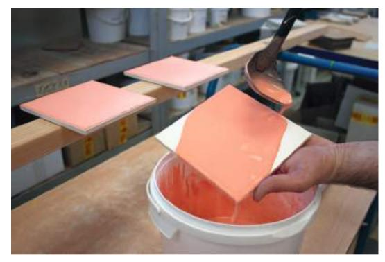
The glaze is ladled by hand onto the bisque – tile for tile.
