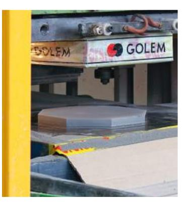
Clay granulates are pressed to tile bodies under high pressure.
