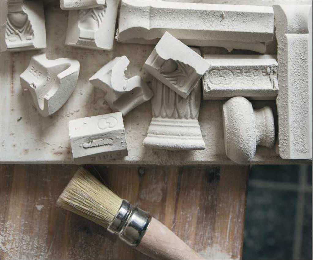
**R**egarding borders, we distinguish between pure profile forms and plastically worked ornaments with flowers, bands and graphic patterns. Due to their protruding, plastic shape, all those pieces are cast with liquid clay into plaster moulds. After drying the burrs are taken off and the surface is sanded down. Subsequently, the border is fired for the first time, the so-called bisque firing.
